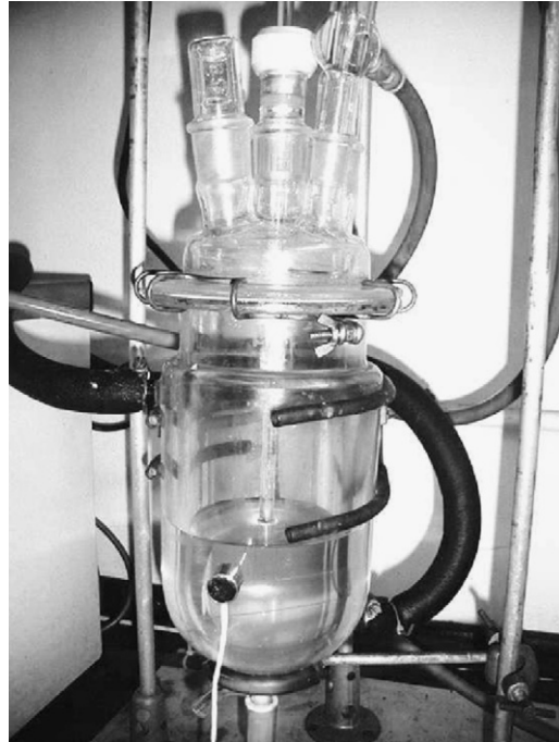
Fig. 8. The multi-particle experimental set-up for itaconic acid stirred in toluene. Tables 1 and 2 contain typical parameter values.
